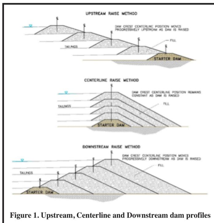
Figure 1. Upstream, Centerline and Downstream dam profiles
